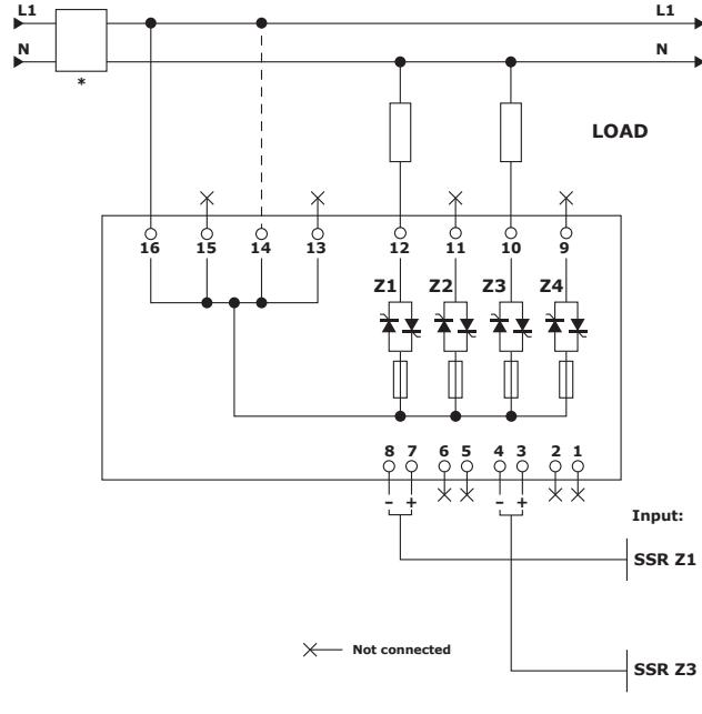
**Diagram of control connection 2x7A - 480V**
