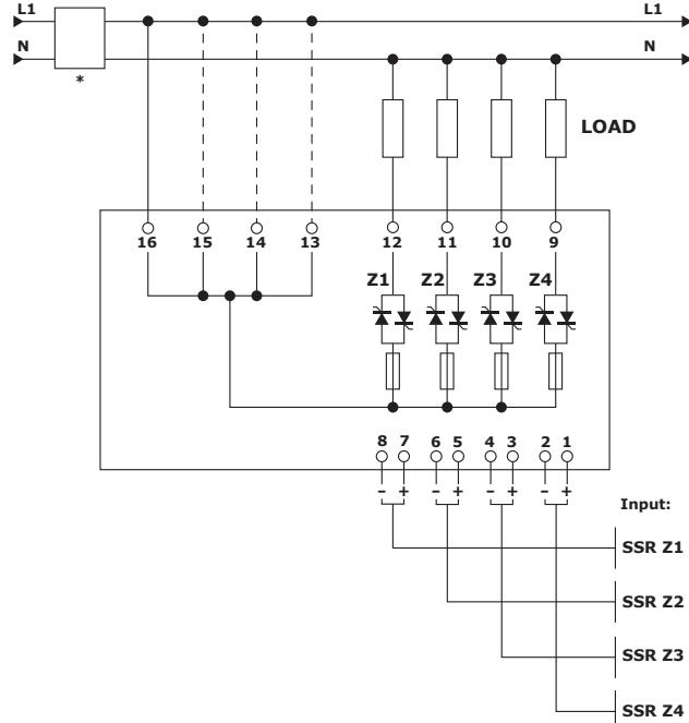
**Diagram of control connection 4x3,5A - 480V**
