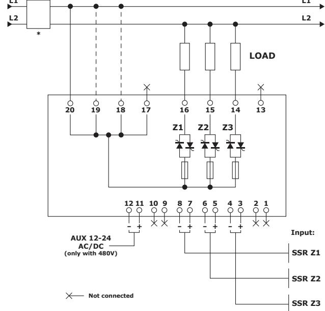
**Diagram of control connection 2x7A - 230V**
