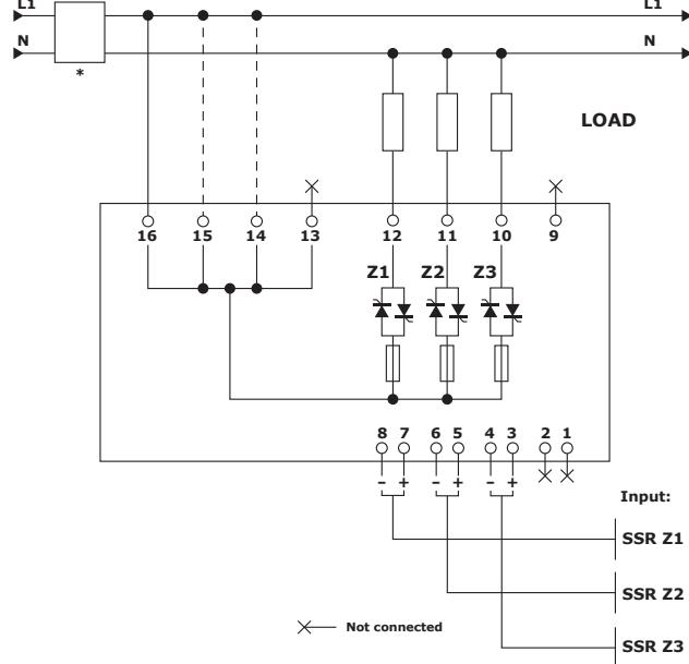
**Diagram of control connection 3x4,5A - 480V**
