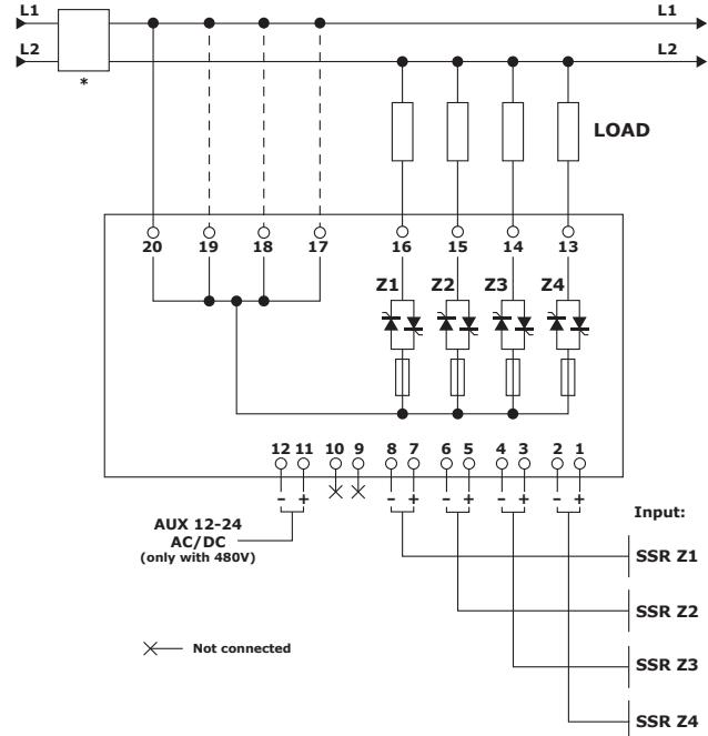
**Diagram of control connection 3x4,5A - 230V**
